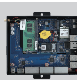
SOM based Mainboard (Compact CPU Board + I/O Board)
